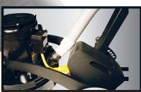
A 2" vacuum port and variable-position positive lock handle are standard on this floor machine.
